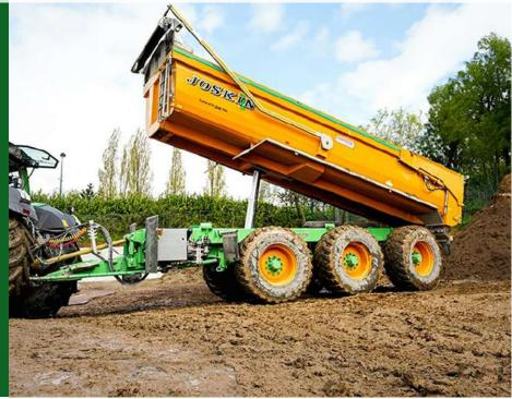
The new JOSKIN Trans-KTP-24/54 can carry up to 24 tonnes of technical load in its 13 m<sup>3</sup> body. Slightly tapered, it is made of Hardox 450 steel and is 105 cm high. The 8 cm wider rear than the front makes sure the contents of the trailer flow out freely. The chassis of the Trans-KTP 24/54 is 700 mm wide, allowing the body to be fitted with wide tires (max. 666 mm) without exceeding the 255 cm width limit required in some fields of activity.
